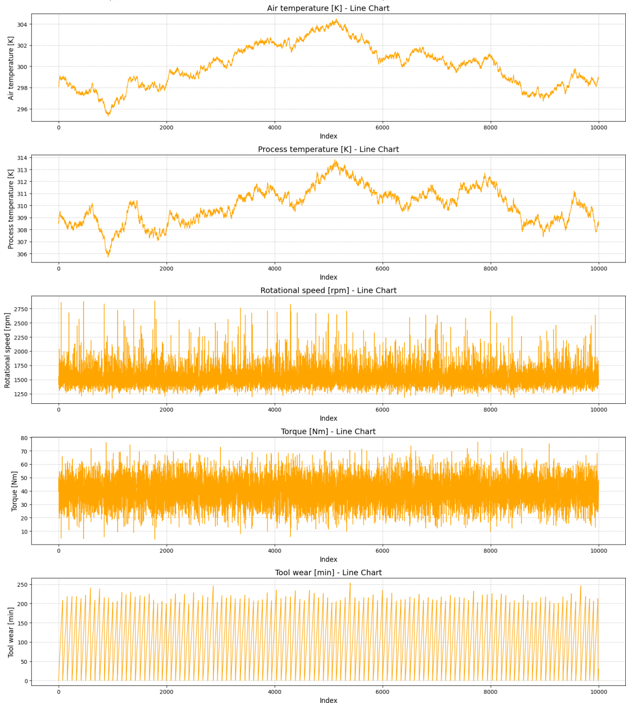
Figure 6 Line charts of sensor variables (air temperature, process temperature, rotational speed, torque, and tool wear)
