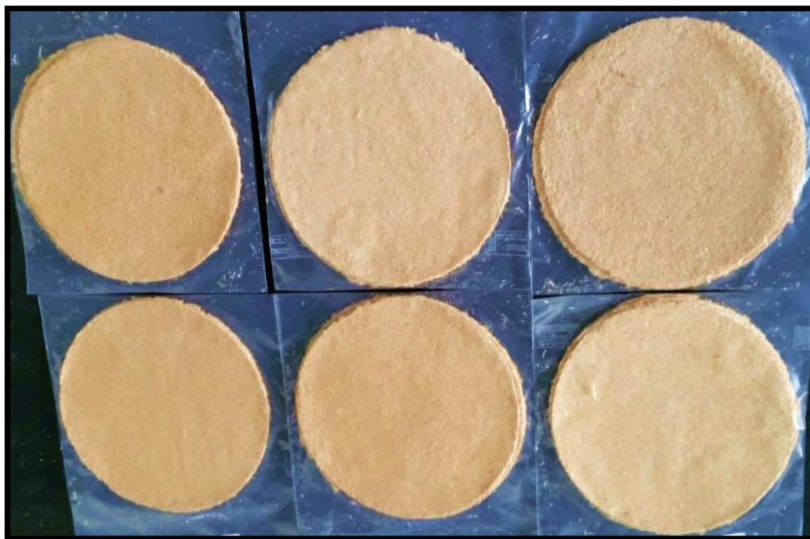
Fig. 10: Handmade paper by varying concentration of binding agent (gum rosin) in sugarcane bagasse
