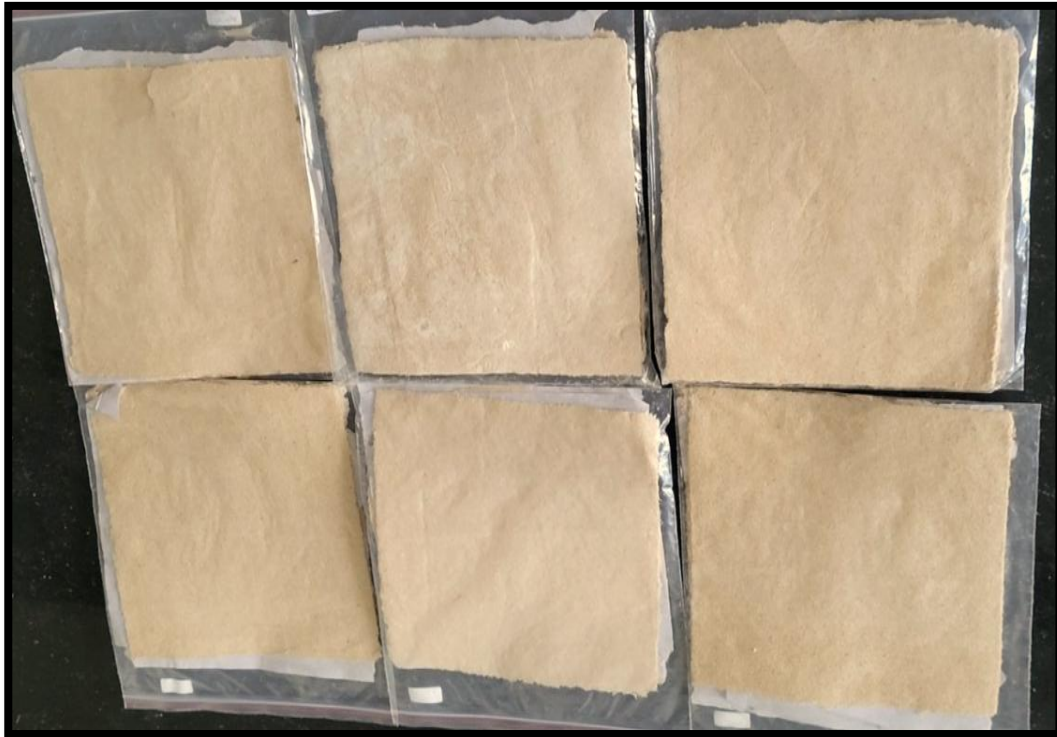
Fig. 3: Handmade paper by varying concentration of binding agent (starch) in rice straw
