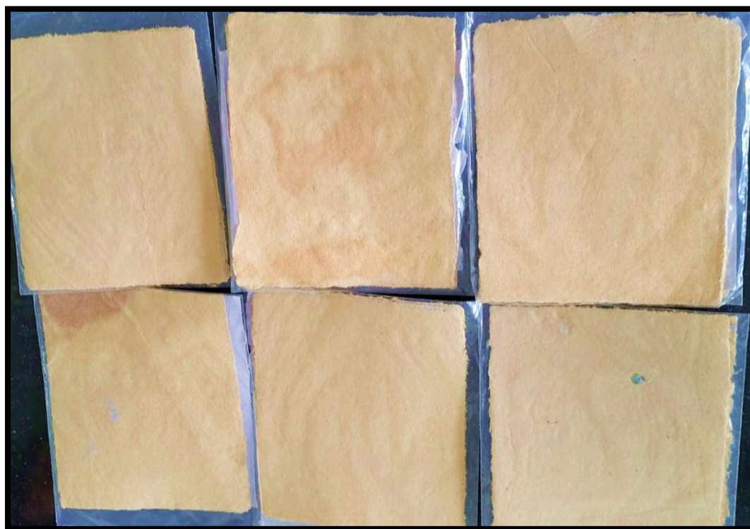
Fig. 6: Handmade paper by varying concentration of binding agent (gum rosin) in rice straw
