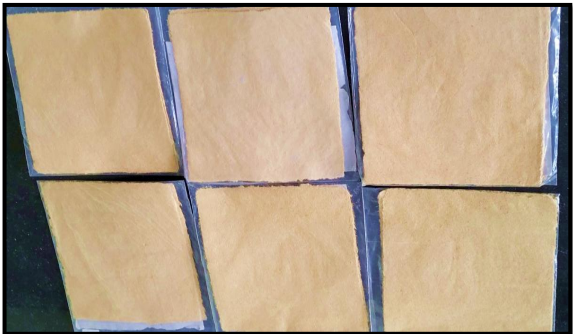
Fig.5: Handmade paper by varying concentration of binding agent (corn flour) in rice straw
