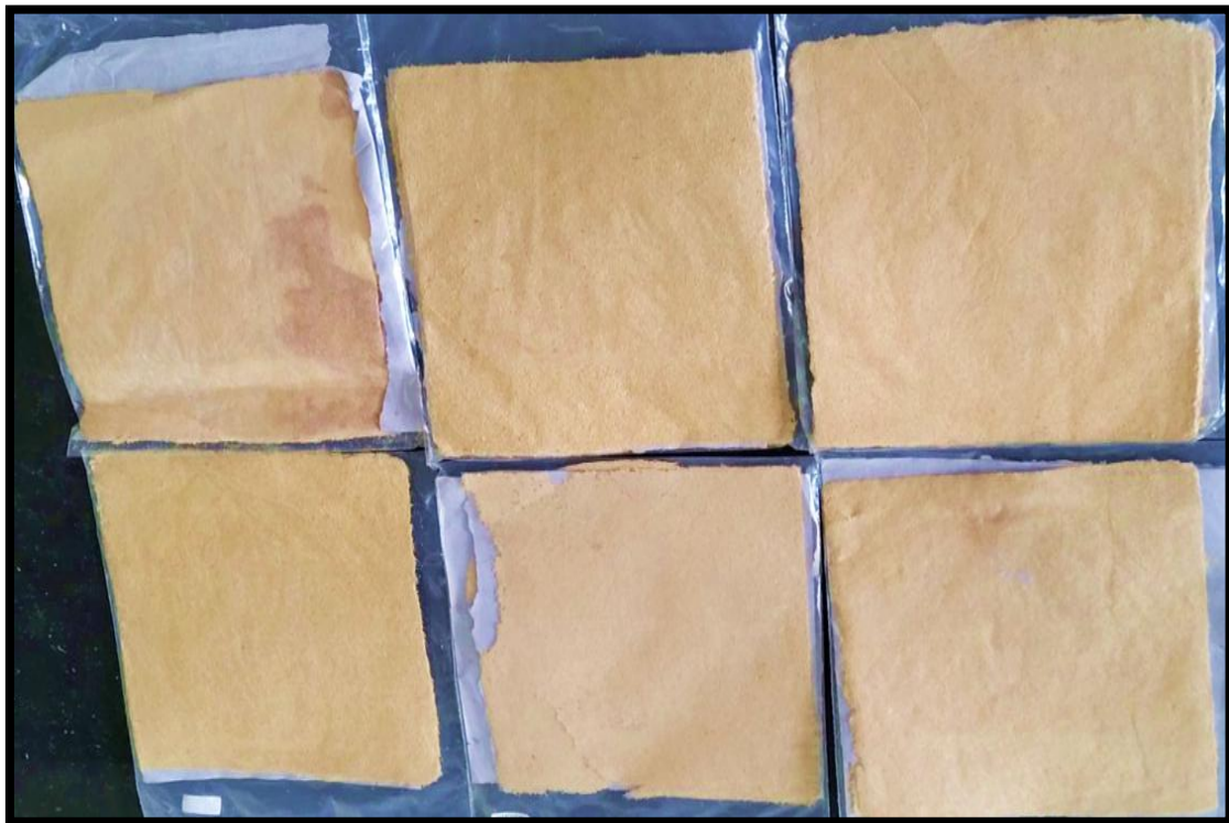
Fig. 4: Handmade paper by varying concentration of binding agent (aloevera) in rice straw
