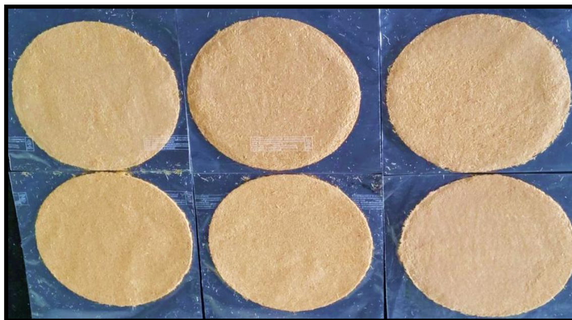
Fig. 9: Handmade paper by varying concentration of binding agent (corn flour) in sugarcane bagasse
