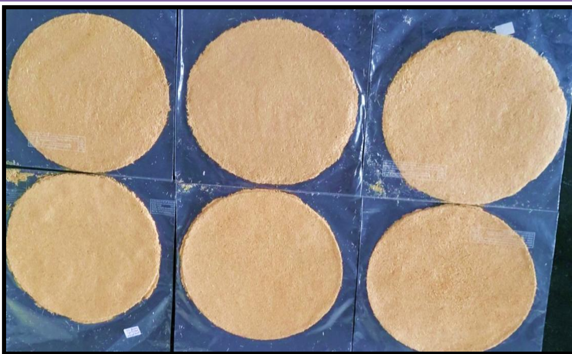
Fig. 7: Handmade paper by varying concentration of binding agent (starch) in sugarcane bagasse
