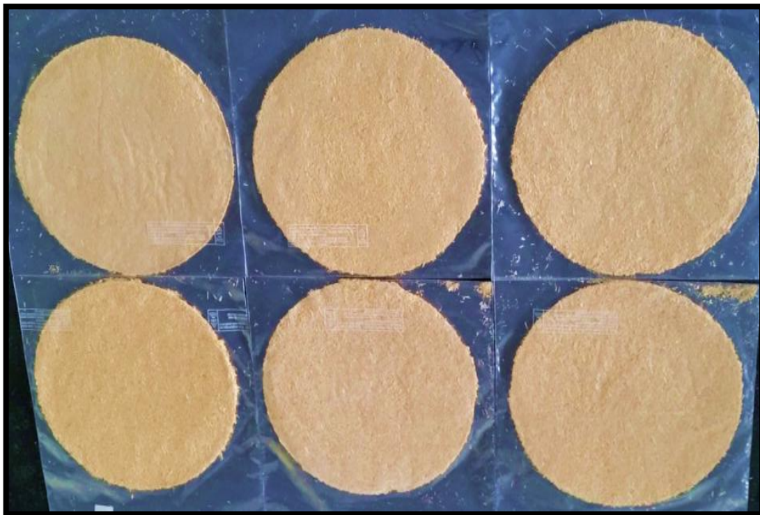
Fig. 8: Handmade paper by varying concentration of binding agent (aloe vera) in sugarcane bagasse
